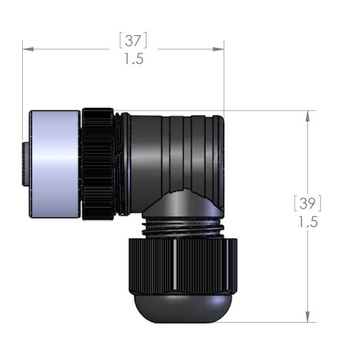
All connections made via Screw Terminals.
