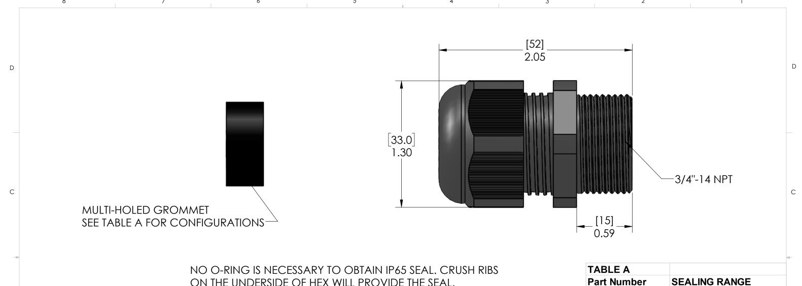
ON THE UNDERSIDE OF HEX WILL PROVIDE THE SEAL.
