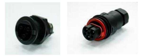
The RS PRO series of waterproof power connectors are ruggedly built connectors sealed to an IP67 rating with a push-lock coupling which requires the series coupling tool to remove. This provides a more secure connection ideal for use when electrical safety or tampering may be an issue. The M25 range of connectors are designed with 3 gold plated contacts rated to 30A at 600V and are available in panel to cable or cable to cable variations. Features & Benefits:
