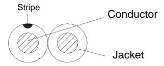
Cable Marking: RS PRO 2 Core × 0.4 mm<sup>2</sup> Speaker Cable 60V
