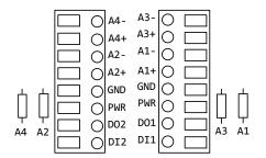
Ax+ and Ax–. Analog IN x. Analog inputs for devices requiring more than one connection, such as thermocouples or RTDs. When there is no Ax–, use Ax+ as an analog input. DIx. Discrete IN x DOx. Discrete OUT x GND. Ground/DC common connection
