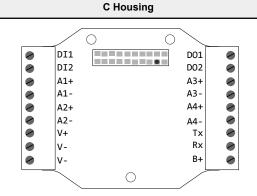
B+. 3.6 V DC to 5.5 V DC (use for battery powered models only) RX/-. Serial communication line for the Gateway. No connection for Nodes
