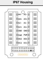
Ax+ and Ax-. Analog IN x. Analog inputs for devices requiring more than one connection, such as thermocouples or RTDs. When there is no Ax-, use Ax+ as an analog input. DIx. Discrete IN x DOx. Discrete OUT x GND. Ground/DC common connection PWR. 10 V DC to 30 V DC power connection
