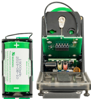
Figure 5. Battery pack and board
