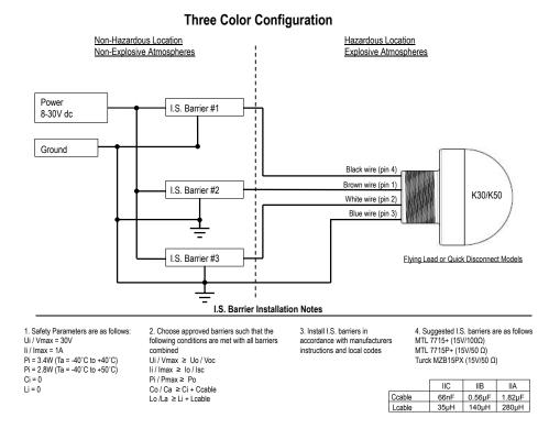
Figure 3. Control Drawing 3-Color Configuration
