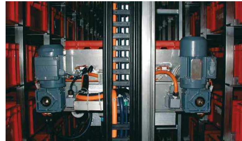
Control cable Chainflex® CF10 in storage and retrieval units for high-bay warehouses. E-Chain®. System E2
