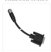
Cordset A-Code M12 to D-SUB Double Ended 17-Pin Straight Female; 25-pin Straight Male Connectors with Shield 1.00 m (3.28 ft) in Length Black PVC Jacket, Nickel-Plated Brass Nut Part Number: 806015
