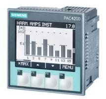
SENTRON, measuring device, 7KM PAC4200, LCD, L-L: 500 V, L-N: 289 V, 5 A, 3-phase, Modbus TCP, optional Modbus RTU / PROFINET / PROFIBUS / DI/DO, apparent/active/reactive energy / cos phi, harmonics: 2.-64., THD, class 0.2 acc. to IEC61557-12 or cl. 0.2S acc. to IEC62053-22, ext-low volt. pwr sup. unit DC, screw terminals
