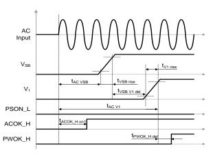
NOTE: AC short dips means below 10 ms; AC long dips means 10 ms to 100 ms
