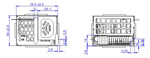
Figure 16. Front and Rear View
