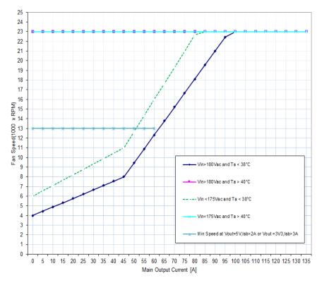
Figure 13. Fan speed vs. main output load
