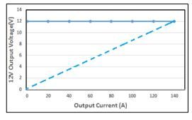
Figure 6. Current Limitation on  $V_1$  ( $V_i = 230 \text{ VAC}$ )
