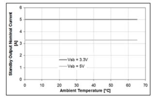
Figure 8. Current Limitation and Temperature Derating on 3.3 / 5  $V_{\rm SB}$
