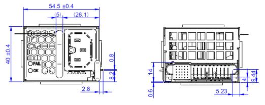
Figure 20. Front and Rear View
