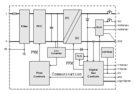
Figure 1. PFE1500 Series Block Diagram
