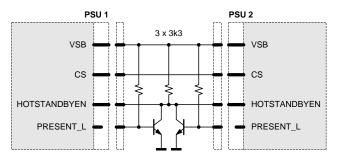
Figure 9. Recommended hot-standby configuration
