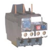
The Telemecanique TeSys D-Line Class 20 Overload Relay provides a motor control solution for longer acceleration times. As a Class 20 overload relay, the unit trips in 20 seconds when the current is 6 times the lowest setting of the relay. The new relays are designed for direct mounting on TeSys D-Line contactors ranging from 9 to 32 amps.
