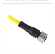
Cordset A-Code M12 Single Ended 5-pin Straight Female Connector 30.48 m (99.97 ft) in Length Yellow PVC Jacket, Nickel-Plated Brass Nut Part Number: 71465
