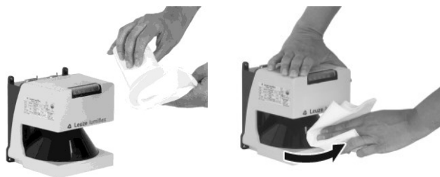
Figure 5-3. Front screen cleaning procedure
