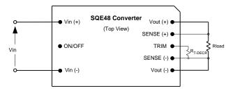
Figure D. Configuration for decreasing output voltage.
