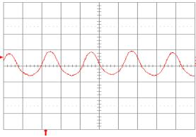
Fig. 13: Input reflected ripple current, i<sub>c</sub> (100 mA/div.), measured at input terminals at full rated load current and Vin = 48 V. Refer to Fig. 12 for test setup. Time scale:  $1 \mu s/div.$
