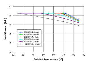
Fig. 2: Available load current vs. ambient air temperature and airflow rates for converter with G height pins mounted horizontally with air flowing from pin 1 to pin 3 and maximum FET temperature ≤ 120 °C, Vin = 48 V.
