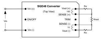
Figure B. Remote sense circuit configuration.
