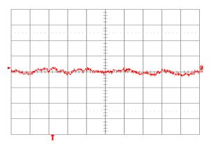
Fig. 14: Input reflected ripple current, i<sub>s</sub>(10 mA/div.), measured through 10 μH at the source at full rated load current and Vin = 48 V. Refer to Fig. 12 for test setup. Time scale: 1 μs/div.
