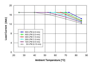
Fig. 1: Available load current vs. ambient air temperature and airflow rates for converter with G height pins mounted vertically with air flowing from pin 1 to pin 3 and maximum FET temperature ≤ 120 °C, Vin = 48 V.
