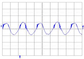
Fig. 11: Output voltage ripple (20 mV/div.) at full rated load current into a resistive load with  $Co = 10 \,\mu F$  tantalum +  $1 \,\mu F$  ceramic and Vin = 48 V. Time scale:  $1 \,\mu s$ /div.
