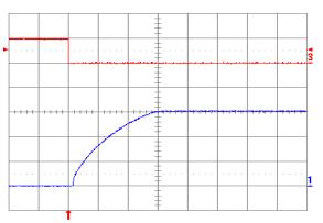
Fig. 8: Turn-on transient at full rated load current (resistive) plus 10,000 μF at Vin = 48 V, triggered via ON/OFF pin. Top trace: ON/OFF signal (5 V/div.). Bottom trace: output voltage (2 V/div.). Time scale: 5 ms/div.
