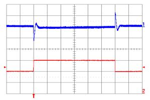
Fig. 10: Output voltage response to load current step-change (10 A – 15 A – 10 A) at Vin = 48 V. Top trace: output voltage (100 mV/div.). Bottom trace: load current (5 A/div.). Current slew rate: 5 A/μs. Co = 470 μF POS + 1 μF ceramic. Time scale: 0.2 ms/div.
