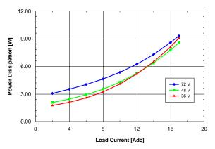
Fig. 5: Power dissipation vs. load current and input voltage for converter mounted vertically with air flowing from pin 1 to pin 3 at a rate of 300 LFM (1.5 m/s) and Ta = 25 ℃.
