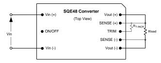
Figure C. Configuration for increasing output voltage.
