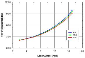
Fig. 6: Power dissipation vs. load current and ambient temperature for converter mounted vertically with Vin = 48 V and air flowing from pin 1 to pin 3 at a rate of 200 LFM (1.0 m/s).
