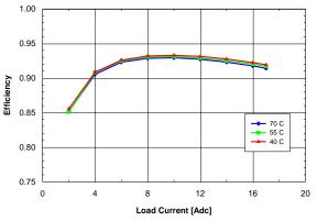
Fig. 4: Efficiency vs. load current and ambient temperature for converter mounted vertically with Vin = 48 V and air flowing from pin 1 to pin 3 at a rate of 200 LFM (1.0 m/s).
