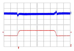
Fig. 9: Output voltage response to load current step-change (10 A – 15 A – 10 A) at Vin = 48 V. Top trace: output voltage (100 mV/div.). Bottom trace: load current (5 A/div.). Current slew rate: 0.1 A/µs. Co = 1 µF ceramic. Time scale: 0.2 ms/div.
