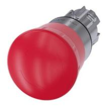
EMERGENCY STOP mushroom pushbutton, 22 mm, round, metal, shiny, red, 40 mm, positive latching, acc. to EN ISO 13850, rotate-to-unlatch, with laser labeling, symbol number according to ISO 7000 or IEC 60417
