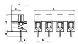
The plug-in terminal strip 322-FBG with a pitch of 10 mm is equipped with a solder pin and designed for the use on PCBs. Due to large pitch and moulding shape, this version is also well suited for applications using higher voltages.
