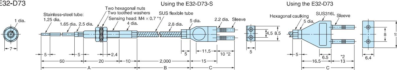
Note: The maximum allowable temperature for section A and B are 200°C. and 110°C. respectively. The section inserted into Amplifier unit (indicated by \*2), however, must stay within the Amplifier Unit's operating temperature range.
