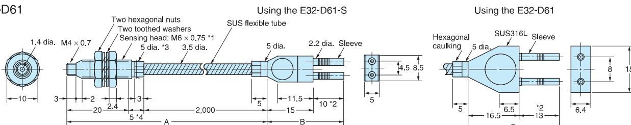
Note: The maximum allowable temperature for section A and B are 200°C. and 110°C. respectively. The section inserted into Amplifier unit (indicated by \*2), however, must stay within the Amplifier Unit's operating temperature range.
