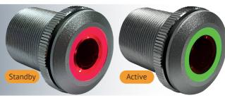
The CTL-SW is a touchless infrared proximity switch, which sits inside a Ø22mm natural anodised aluminium shell. Easily and reliably activated without contact, this proximity switch has a pre-set\* detection range of 4cm. The CTL-SW has onboard LED's showing red when the switch is in standby and green when activated. The momentary action is pre-set\* to 10 seconds.
