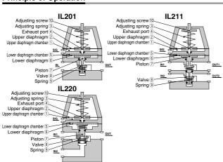
The signal air pressure enters the upper diaphragm chamber ① to generate a force. When this force is larger than the force generated by compressing the adjusting spring ③, the upper diaphragm ② is pushed up, the exhaust port ④ is closed, and the signal air pressure enters the lower diaphragm chamber ⑤ and acts the lower diaphragm ⑥. This pushes down the oiston ⑦ to open the valve.
