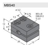
Fixing clamp; material mounting block: Anodized aluminium
