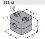
6901321 Mounting clamp for smooth and threaded barrel sensors; material: Polypropylene
