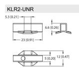
Mounting bracket for mounting magnetic field sensors on round cylinders
