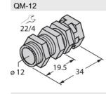
Quick-mount bracket with dead-stop; material: Chrome-plated brass. Male thread M16 × 1. Note: The switching distance of the proximity switches may change when using quick-mount brackets.
