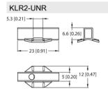
100000596 Mounting bracket for mounting magnetic field sensors on round
