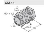
Quick-mount bracket with dead-stop; material: Chrome-plated brass. Male thread M24 × 1.5. Note: The switching distance of the proximity switches may change when using quick-mount brackets.
