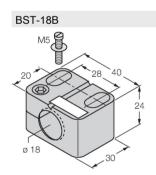
6947214 Mounting clamp for threaded barrel sensors, with dead-stop; material: PA6
