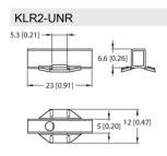
Mounting bracket for mounting magnetic field sensors on round
