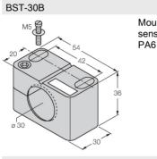
6947216 Mounting clamp for threaded barrel sensors, with dead-stop; material:
