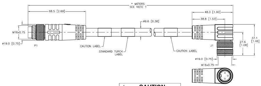
TOLERANCE\* CABLE LENGTH + 4% (OR 50mm) OF LENGTH - 0% (OR 0mm) OF LENGTH WHICHEVER IS GREATER ALL LENGTHS STRIP LENGTH TOLERANCE \* 0-7mm ±0.5mm 8-29mm ±1.0mm ±2.0mm 50-69mm ±3.0mm 70-100mm ±4.0mm ±5.0mm \* UNLESS OTHERWISE SPECIFIED
