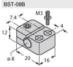
Mounting clamp for threaded barrel sensors, with dead-stop; material: PA6
