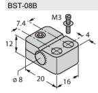
6947210 Mounting clamp for threaded barrel sensors, with dead-stop; material:
