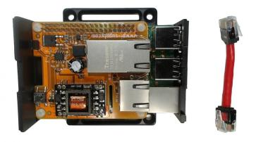
**Step 7** – Connect the Ethernet cable coming from the PoE switch or from the injector.
