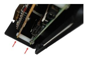
Step 6 - Take the small Ethernet cable and connect it between the Raspberry Pi and the Pi PoE.
