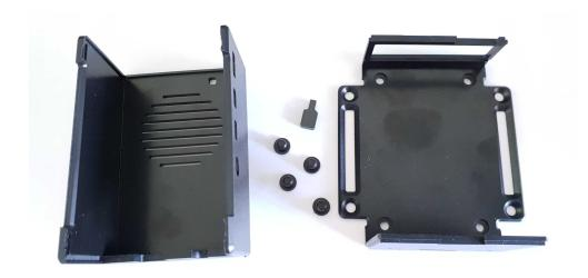
Step 2 - Insert the plastic button extender through the hole of the top part of the case..
