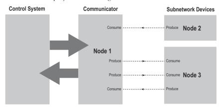
In the figure above, the Communicator 'consumes' data that is 'produced' by a node on the subnetwork. This 'consumed' data can then be accessed from the higher level network. This also works the other way around; the data received from the higher level network is used to 'produce' a message on the subnetwork to be 'consumed' by a node.
